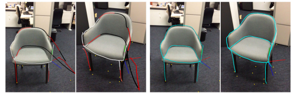
Fig. 15. Drawing multiple curves along a chair (5 strokes; 2.4 mins including 0.3 mins for drawing and 2.1 mins for correction). The left two are the results by ARKit in two views. The right two are our interactive editing results.
